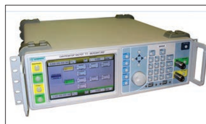
▲ Fig. 7 BELSYNTH signal generator provides two independent signal outputs from 10 MHz to 20 GHz.
