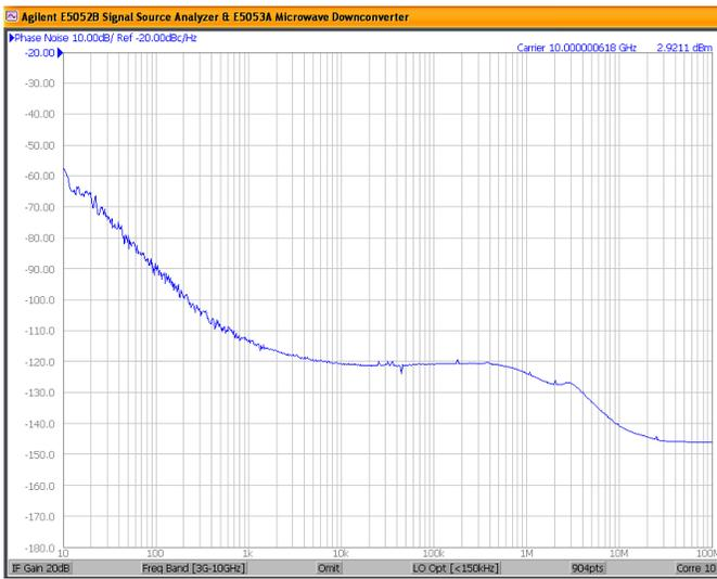
Figure 7. Phase noise at 10 GHz.
