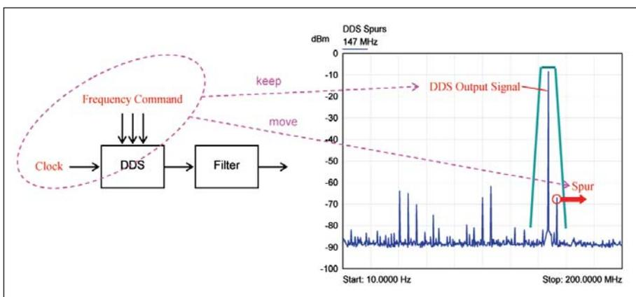
Figure 43 · DDS spur filtering.
