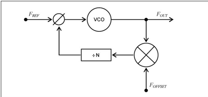
Figure 44 · Frequency mixing within RF feedback path.
