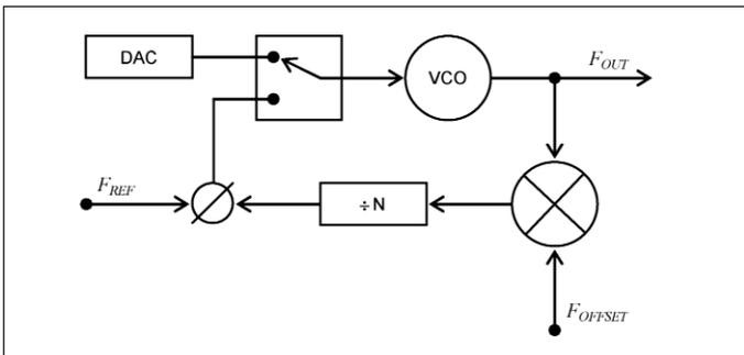
Figure 46 · Initial frequency acquisition.
