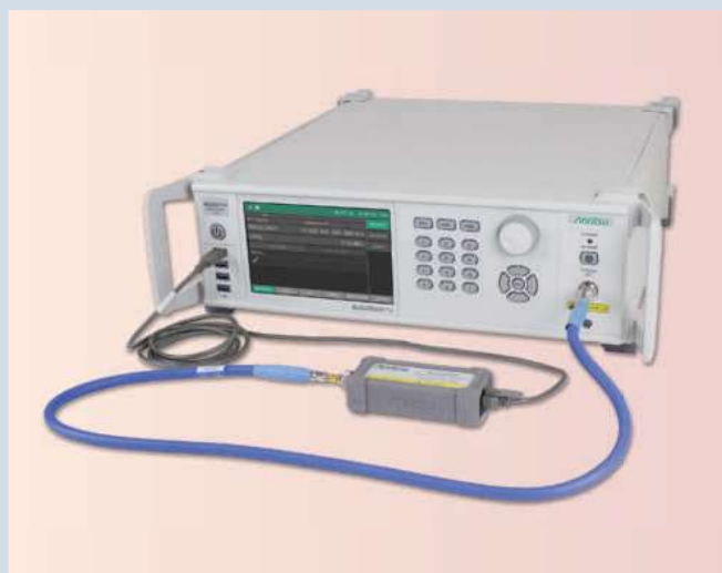
▲ Fig. 3 In-field power calibration with a USB power sensor.
